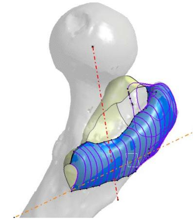
Figure 8. Reverse modeling of trochanteric wedge
