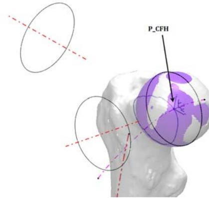
Figure 4. Construction of center of femoral head: P\_CFH
